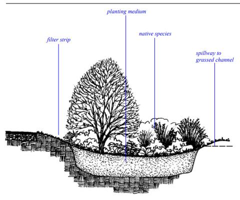
bypasses the facility. To reduce the possibility of clogging by fine sediments, stormwater can pass through a grass filter prior to entering the bioretention area. If stormwater flows are concentrated, a dispersion trench is used to slow and spread out flows prior to entering the grass filter. Space limitations may preclude the use of filters or dispersion trenches.
