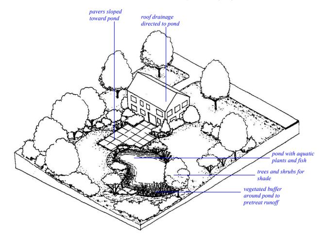
the water temperature, which may affect the fish. Pumps, filters, and other equipment may be needed to maintain proper conditions. The water depth must be at least 15 inches deep to maintain a habitat for the fish during winter. Ornamental ponds and other water features without fish could also be installed but the fish help control any potential mosquito breeding problems.
